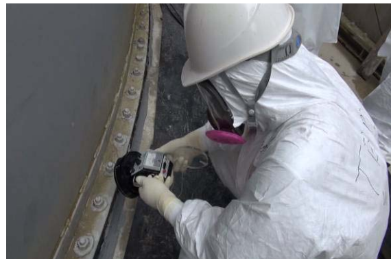
Tank patrol (Geiger counter is used to check for minute leaks from flanges)
