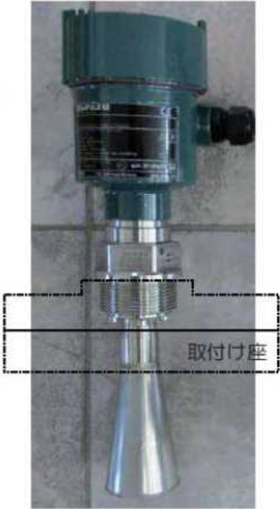
Photo 9 Radar-type water gauge
