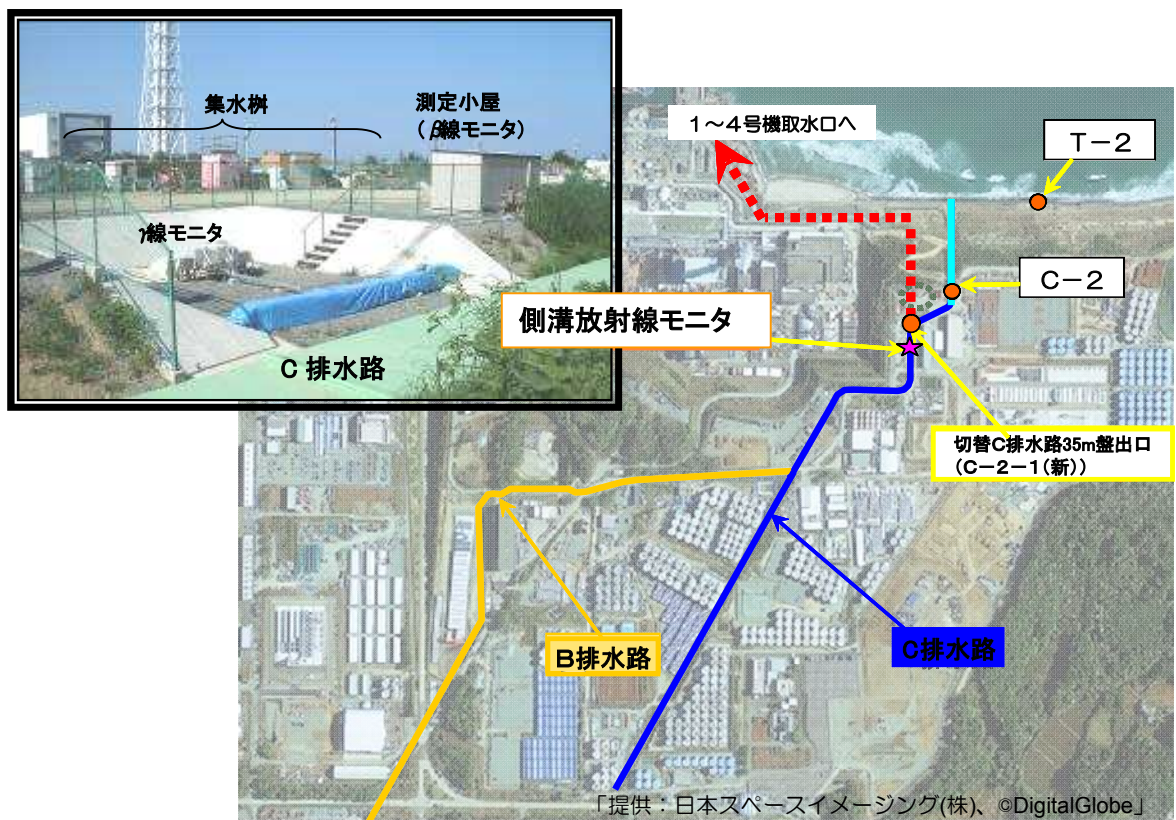
Fig. 8 Diagram showing positions where side ditch radiation monitors installed
