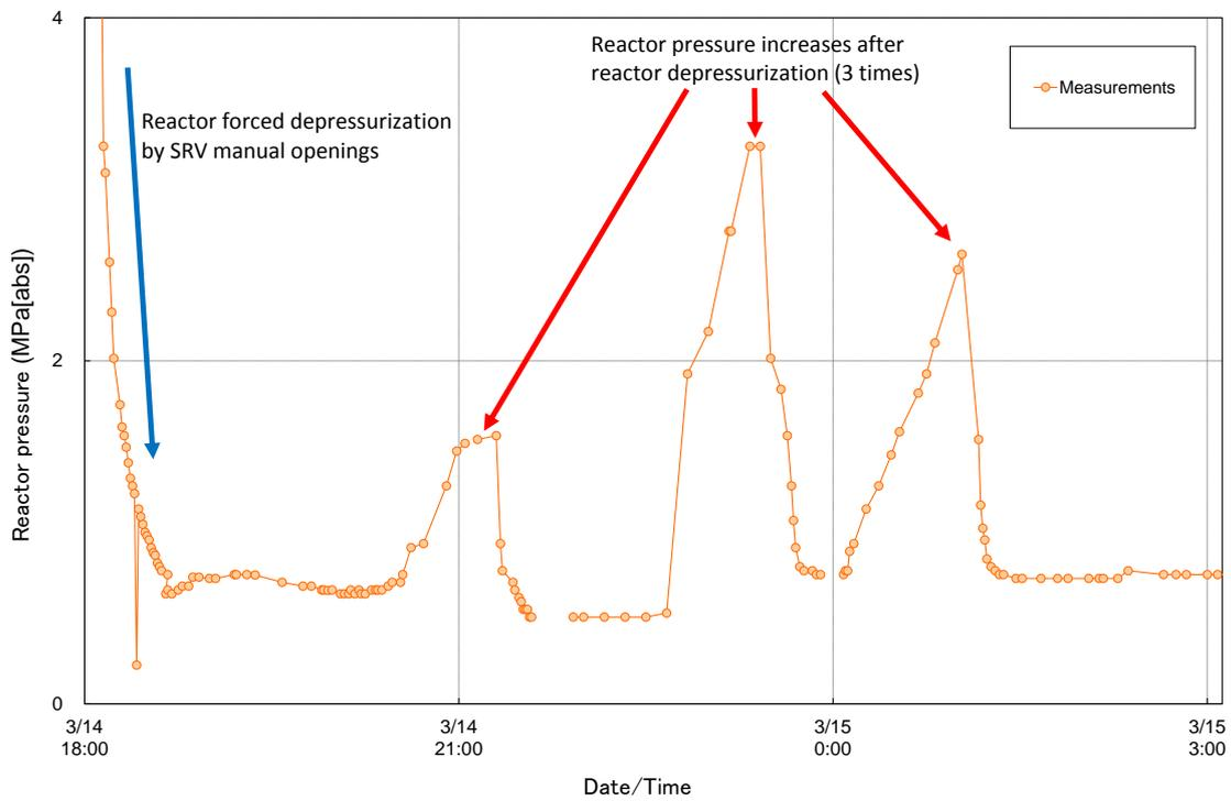
Figure 1 Three reactor pressure increases after reactor depressurization
