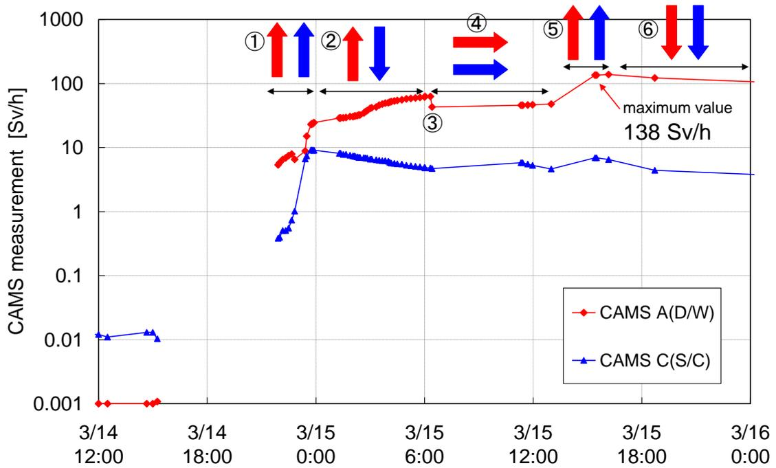
Figure 2 CAMS readings
