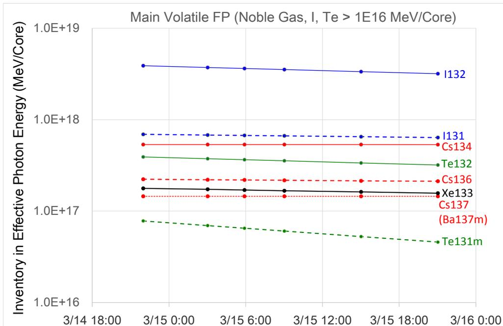
Figure 7 Main volatile FP inventory in the core (in the unit of source energy)
