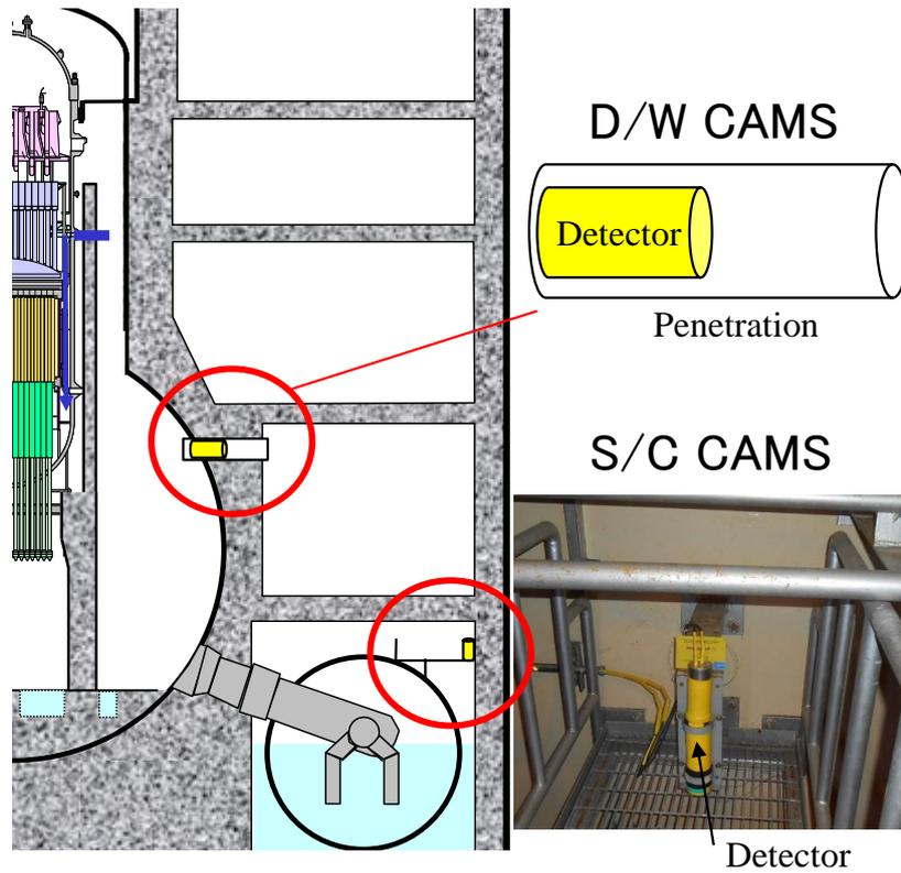
Figure 3 Locations of CAMS detectors in the D/W and S/C
