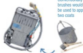
We have developed paint that is highly viscous and does not disperse into the air. The paint is applied using an auto-feed system that enables a single application of a thick coat.
