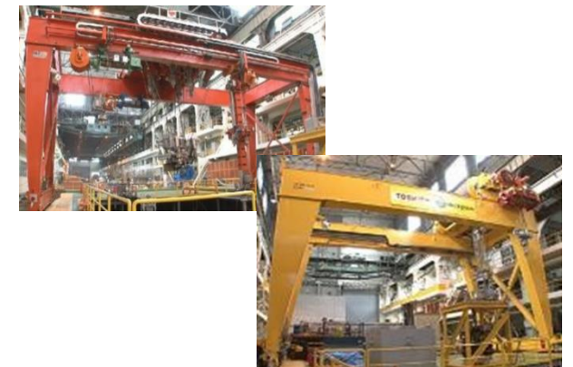
Unit 3 fuel handling machine (top), crane (bottom)
