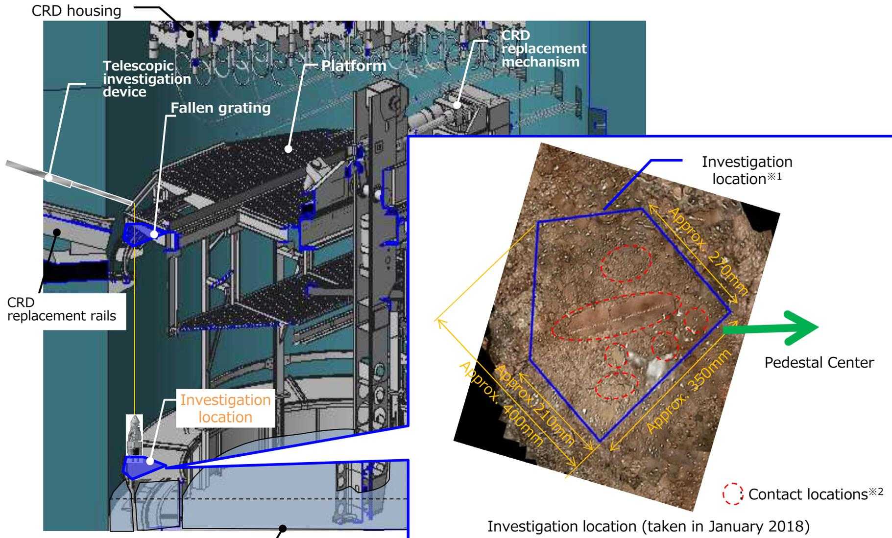
※1 : The range of this internal investigation is shown using a photo taken in January 2018 so field conditions may have changed slightly. (The surface area of the area that can be surveyed is estimated to be approximately 2% of the entire surface area of the bottom of the pedestal (including cable trays))
