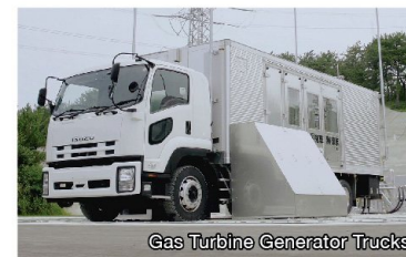
Gas Turbine Generator Trucks
