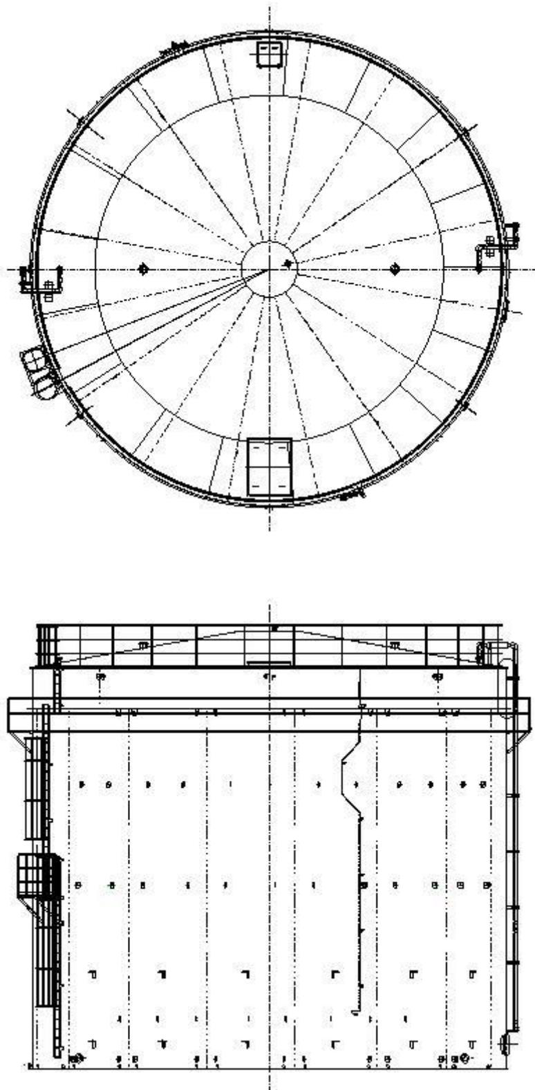
溶接型タンク概略図 (J4(2,900m<sup>3</sup>))
